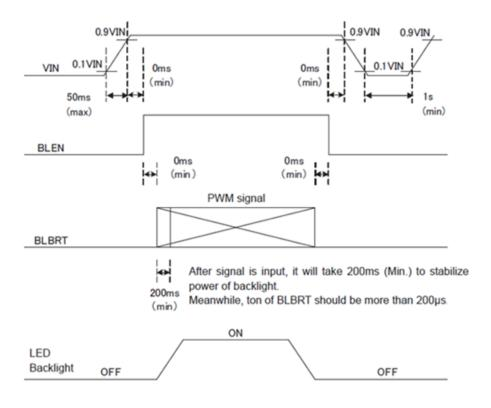
2)  $V_{IN} = 24V$ , Temp. = 25°C,  $D_{PWM} = 100\%$
