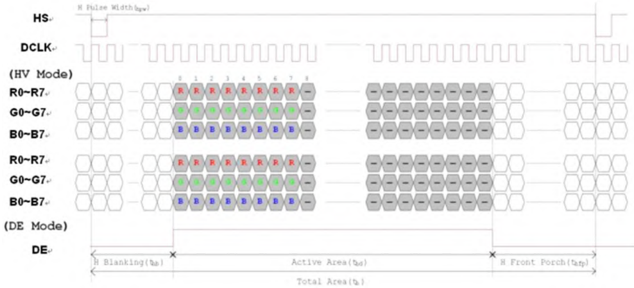
Figure 3. 1 Horizontal input timing diagram.
